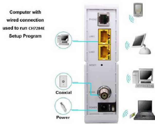
Sample Wireless Network Connections (CH7284E model shown)
